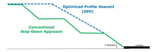
Conventional arrival procedures have multiple segments of level flight during the descent and each step down requires a change in power settings. OPD procedures enable arrival aircraft to descend from cruise altitudes to final approach with significantly fewer level-offs. Typically, this occurs between 30 and 15 nautical miles from the end of the runway. Since aircraft can use lower and steady power settings, OPD procedures can result in reduced fuel burn, lower emissions and reduced noise.
